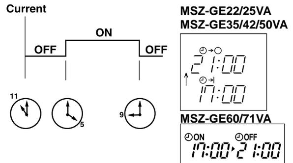
**NOTE:** If the main power is turned OFF or a power failure occurs while ON/OFF timer is active, the timer setting is cancelled. As these models are equipped with an auto restart function, the air conditioner starts operating with timer cancelled when power is restored.
