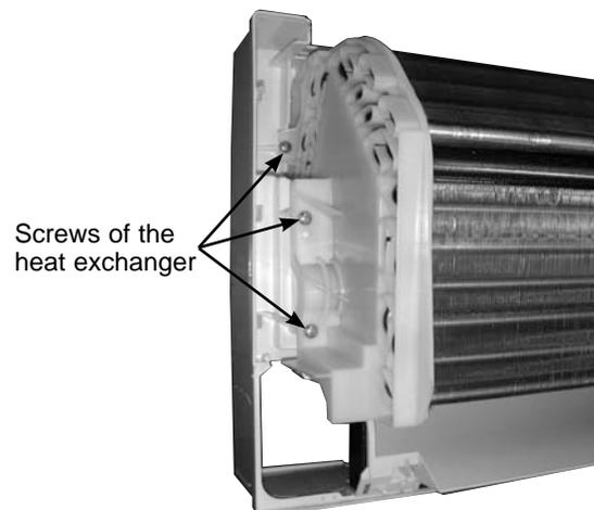
Screws of the heat exchanger
