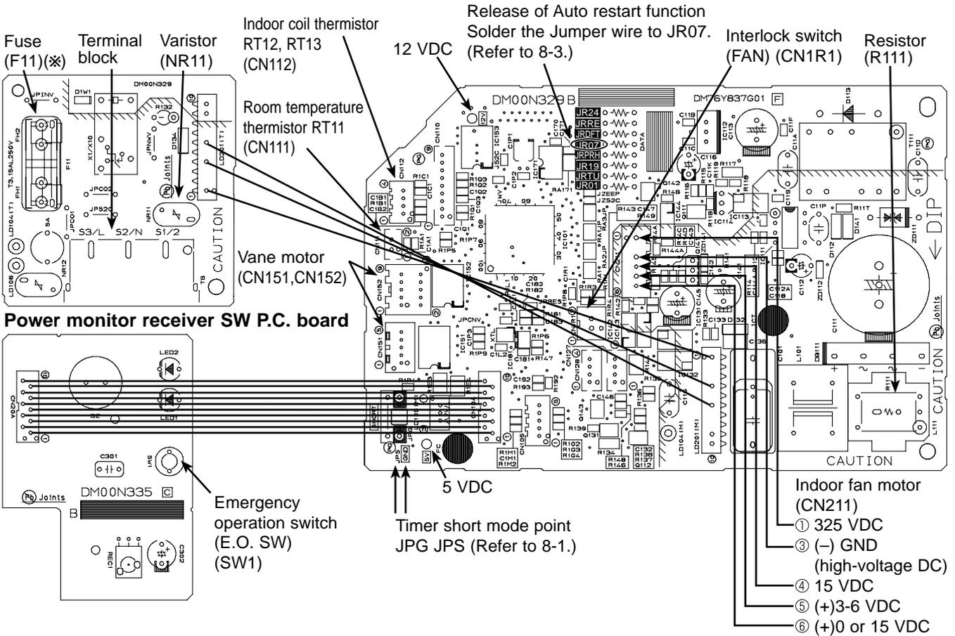
※ Please replace the fuse after removing the indoor terminal P.C. board from the electrical box.
