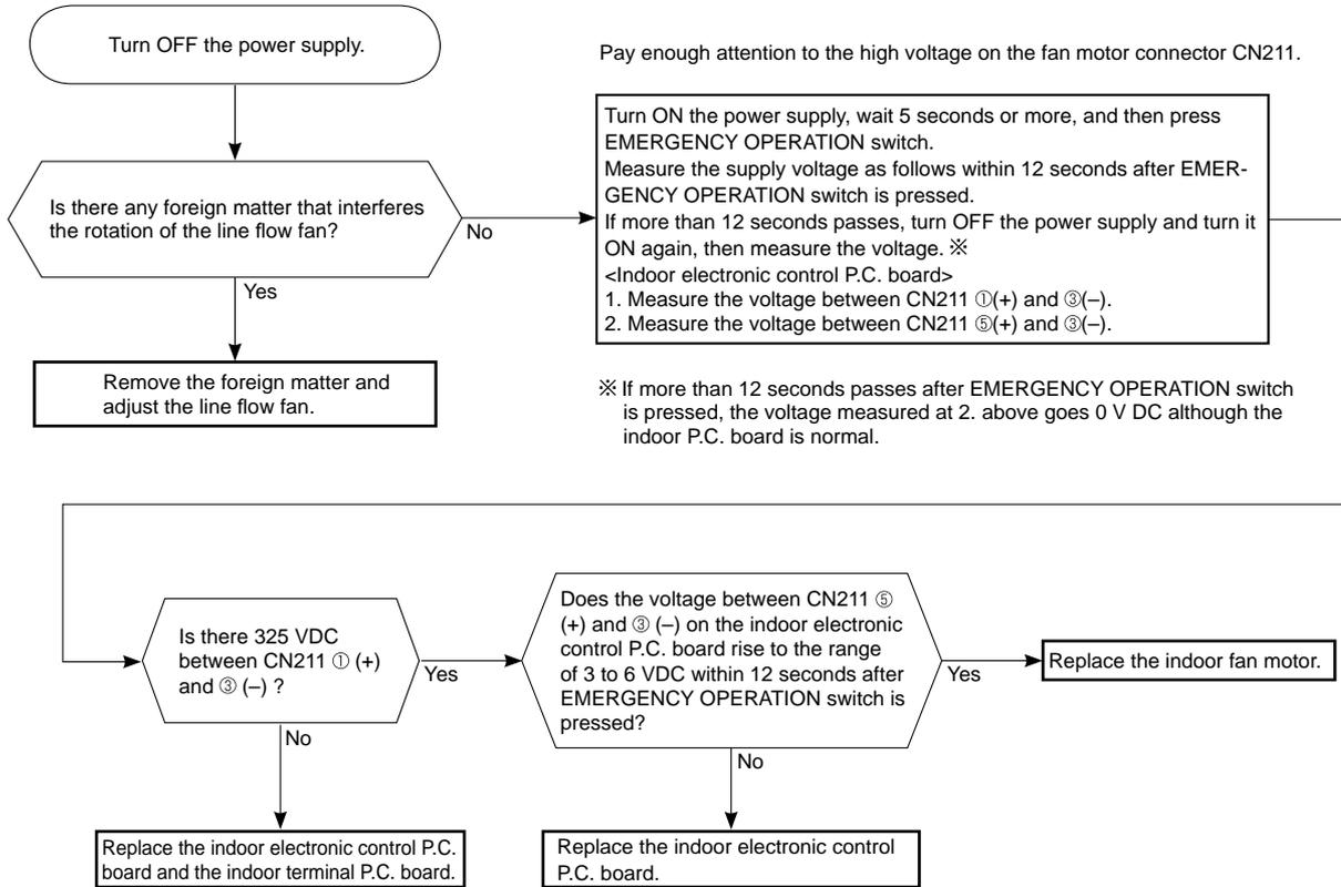
The indoor fan motor error has occurred, and the indoor fan repeats "12-second ON and 30-second OFF" 3 times, and then stops.
