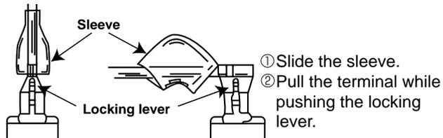
(2) The terminal with this connector has the locking mechanism.
