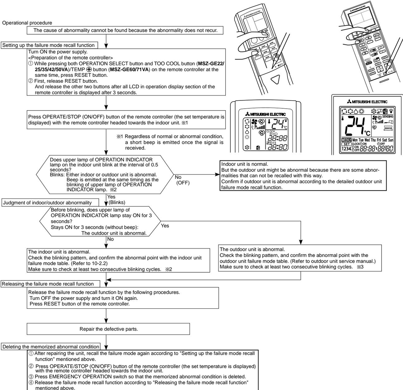
**NOTE:** 1. Make sure to release the failure mode recall function once it is set up, otherwise the unit cannot operate properly.
