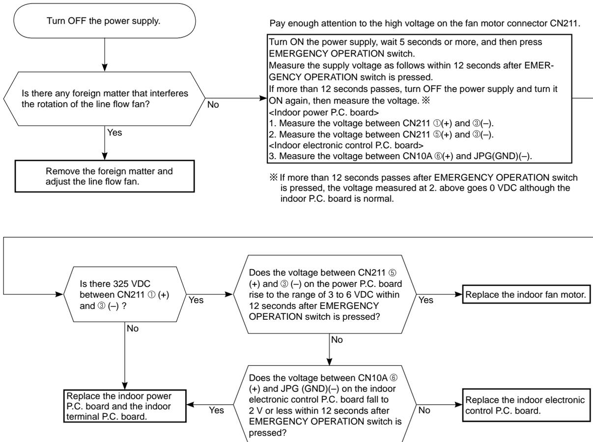
The indoor fan motor error has occurred, and the indoor fan repeats "12-second ON and 30-second OFF" 3 times, and then stops.
